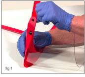
7: Take the visor peak and locate it over the bolt and clear visor. Push on the retaining nut and secure the first hole. Take the remaining bolt and insert it through the last hole of the head strap and visor. Bring across the secondary head strap and push it over the bolt as shown (fig 1). Add the remaining nut to secure all the pieces and push together to fix.
