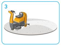
Scrub area to be cleaned, using either scrubbing pad or brushes for textured floors. Double scrub area if heavier soilage.
