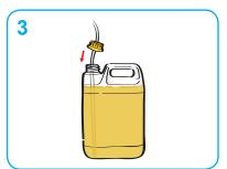
Wearing gloves and goggles insert feeder tube into bottom of container. Screw cap closed.
