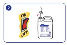
Switch off machine and wearing gloves and goggles remove feeder tube from empty container.
