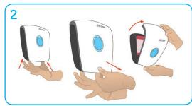
To open the dispenser push the left and right pads underneath, pull out at the bottom and pull the cover down from the top.
